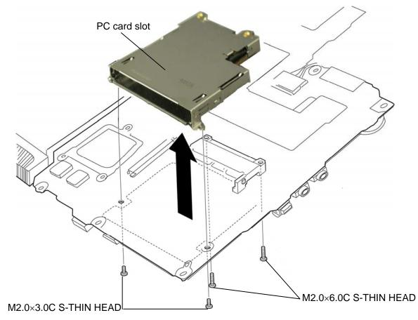
Figure 4-40 Removing the ExpressCard slot
